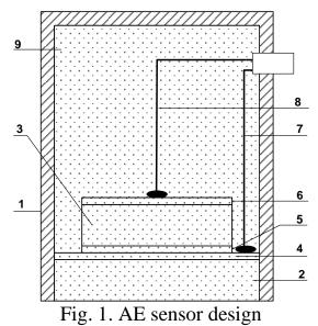
1 - body, 2, 3 - piezoelectric, 4 - a non-working electrode, 5, 6 - working electrodes, 7, 8 - wire, 9 - the body of the damper (a composite of tungsten carbide, titanium nitride and epoxy resin).
