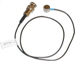
Fig. 2. Exterior view the AE sensor
